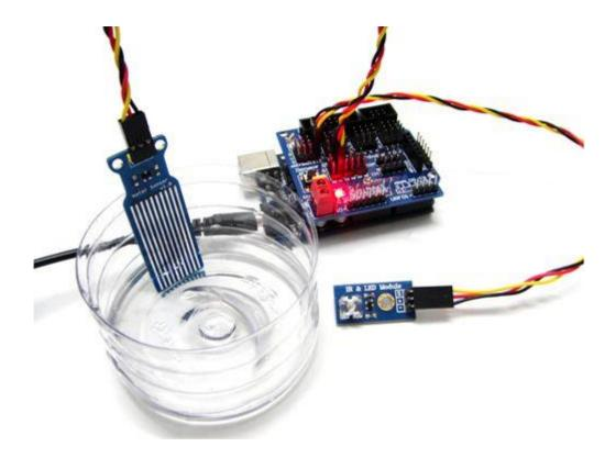
Water level has not reached alarming value, the system will not alarm, LED will not light up.
