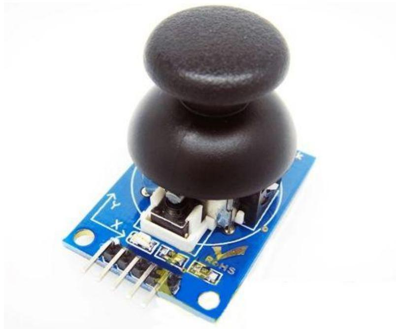
On the principle, the control rod can be considered that it is organized by the two potentiometer and a button
