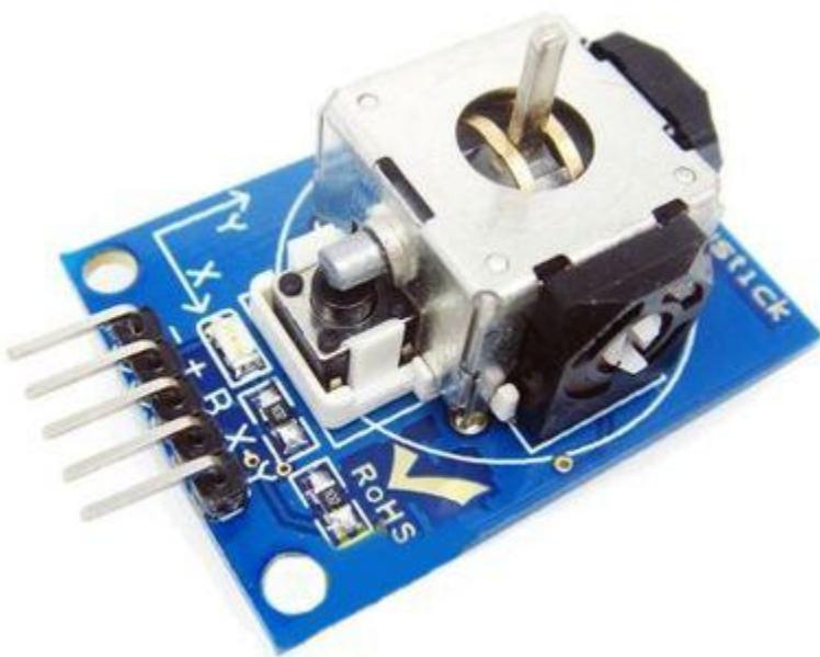
Two of the input value of potentiometer are respectively to show the user offset in the X and Y axis, and the type of offset is analog ; the button is used to show whether the user push down button in the Z axis, its type is the digital quantity. Therefore the control rod contain a total of three input interface which are used to connect X, Y, and Z
